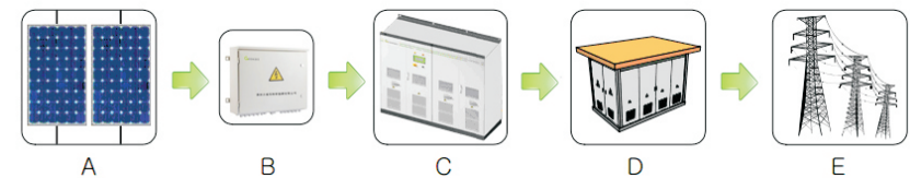
Figure 3-1 Grid-connected PV system
