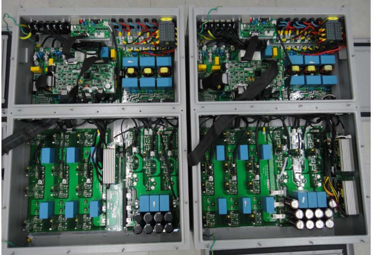
Internal view of the unit: The left photo is model: KSG-30K, KSG-36K-HV, the right photo is model: KSG-50K, KSG-60K, KSG-60K-HV
